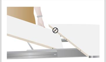
Make sure to open the extension mechanism completely, before inserting the extension leaf/leaves.
